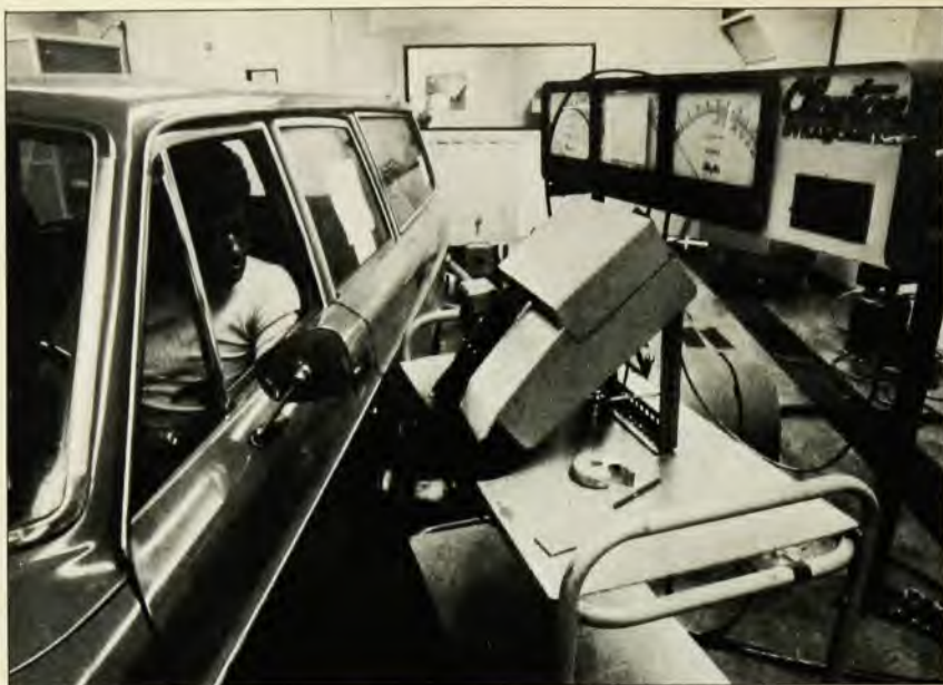
A new car is being tested at the EPA Vehicle Emission Test Center in Ann Arbor, Michigan. Auto makers argue that emission-control devices waste energy. EPA-DOCMERICA photo by Joe Clark.
