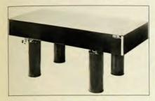
a dense array of tapped holes, or magnetically. The Super-invar series includes tables and breadboards of various sizes and shapes, and modular design permits on-site installation of large or custom configurations.—Newport Research Corp., 18235 Mt. Baldy Circle, Fountain Valley, CA 92708.
