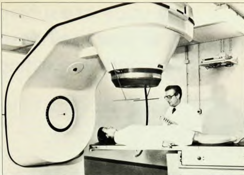
Cyclotron-based neutron-therapy unit , built by the Cyclotron Corporation in Berkeley. Neutron irradiation has been successful in the treatment of malignant tumors. Figure 9
