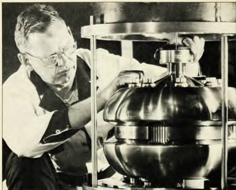
The rotor of a neutron-beam "chopper" is being assembled at Brookhaven. Despite its mass of 350 kg, it can rotate continuously at 15 000 rpm suspended by the thin shaft seen in the photo. The device produces a pulsed neutron beam for nuclear-structure studies.
