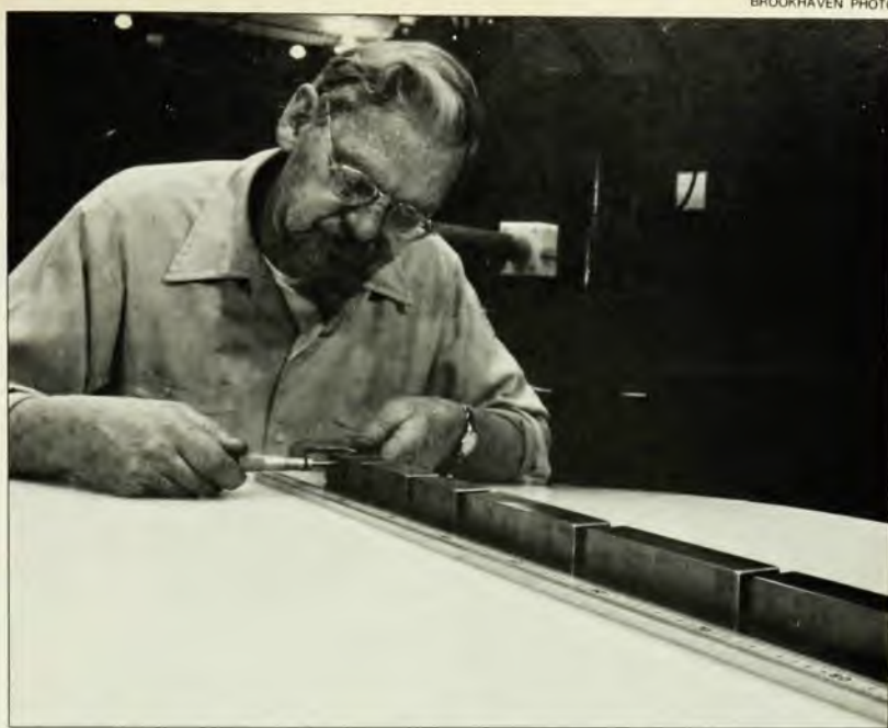
Some 14.5 pounds of isotopically pure iron 56, worth over $660 000, go into making this high-energy neutron-beam filter. Here the carefully machined parts are being checked before insertion into the reactor. To exploit the peculiar property this isotope has of being virtually transparent to neutrons near 25 keV in energy, the iron has been enriched to 99.87% Fe 56 in an electromagnetic mass separator. The filtered beams are for experiments ranging from basic nuclear-structure research to in-vivo analysis of heavy elements in body tissues. Figure 3
