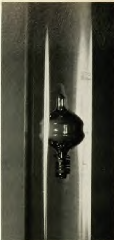
Magnetic buoy levitated in a fluid. The buoy, about 1 cm high, is used to make an accurate measurement of the fluid density. Figure 6
