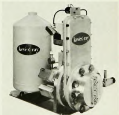
Five X-ray photon detectors are multiplexed to yield exceptionally high data rates. The gate valve removes the beryllium window so that low energy X-rays may be analyzed.
