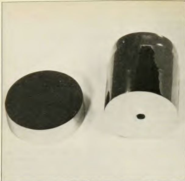
High-purity germanium detectors. The left photograph shows two common detector geometries; on the left is a planar detector that uses the full area of the germanium wafer, and a coaxial detector is on the right. The right photograph shows the heart of a germanium gamma-ray spectrometer. A part of the aluminum heat shield has been removed
