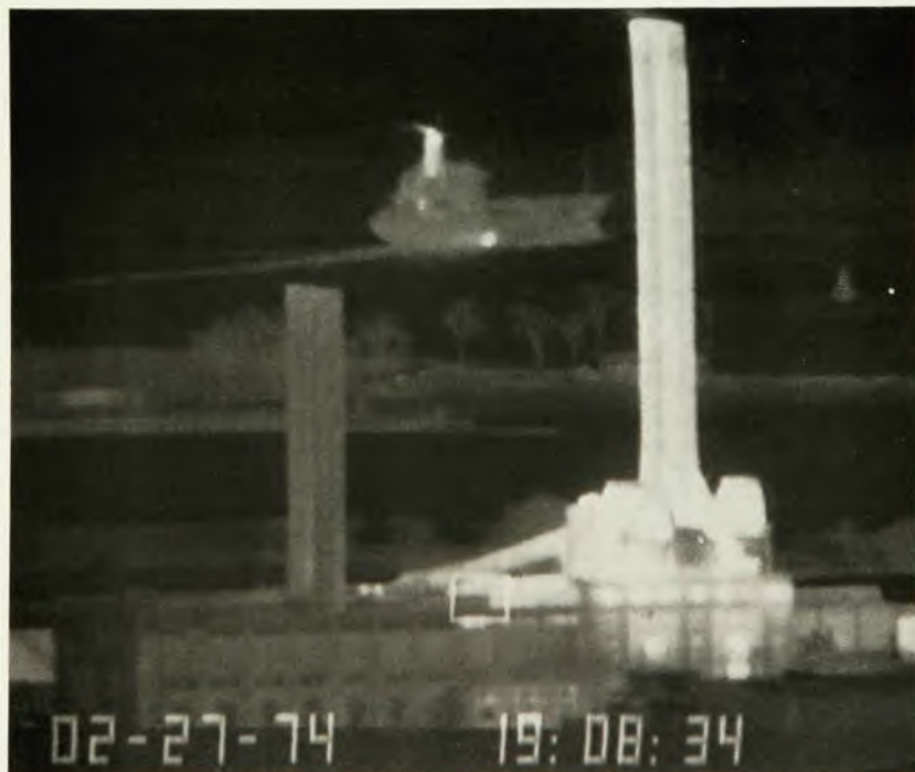
A ship in Boston Harbor taken in darkness from the Prudential Building, using a HgCdTe detector array. The white object in the foreground is a warm smokestack. Photograph supplied by Honeywell Radiation Center, Lexington, Mass.
