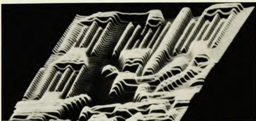
Infrared imagery. The top photograph shows an electrical power station as seen at 11 pm from a plane at 500 feet, using a HgCdTe detector array. Black is cold, white is hot; note that one transformer in the transformer bank is very white, indicating that it is much hotter than the others. The lower photograph is an isometric microimage of a gate circuit, generated by a liquid-nitrogen-cooled InSb detector. Photographs supplied by Texas Instruments Inc, Dallas, Texas (top) and Barnes Engineering Co, Stamford, Conn. (bottom).
