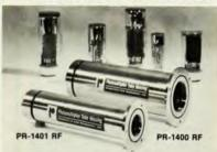
TESTED WITH BROADBAND, HIGH GAIN PHOTON COUNTING SYSTEMS, these high performance PMT housings provide — Electrostatic Shielding at cathode potential, Magnetic Shielding (.040" thick high permeability material) extending ½ cathode diameter in front of photo cathode. Removable Universal Front Mounting Flange allows interchange with most commercial housings.
