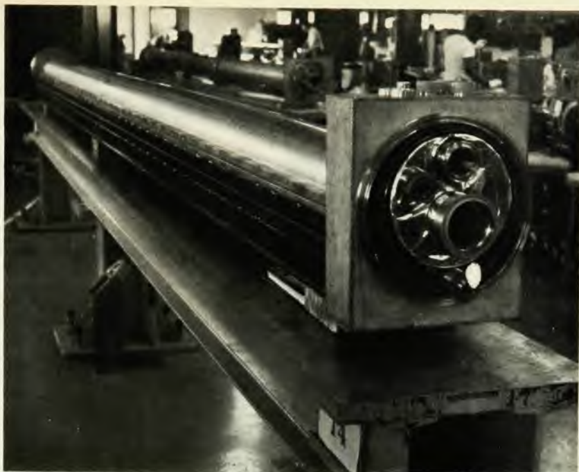
A completed magnet lying on its side in a half core (compare figure 3a). With mass-production techniques at Fermilab these magnets can currently be made in trial production runs at the rate of one a day, a rate that will be quadrupled to meet the goal of constructing the entire Super Ring in a year. Installation is not expected to disrupt the normal operation of the Main Ring; it will be done during the one day each week set aside for maintenance. Figure 4
