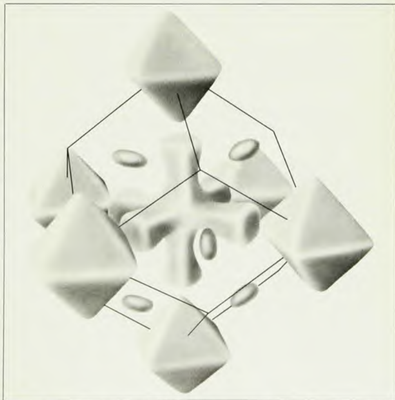
Proposed Fermi surface for bcc tungsten. The structure at the center is an electron pocket, surrounded by hole pockets in zone faces and at corners. From the book, after A. V. Gold.
