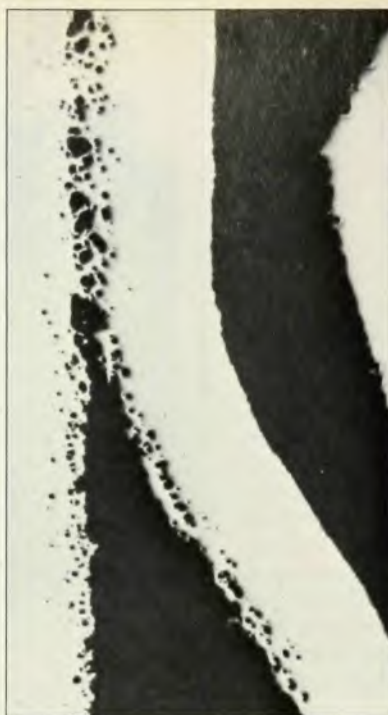
A partial spall (dynamic rupture) is formed by the coalescence of voids in an aluminum plate of commercial purity. The photo on the left represents a width of about 5.0 mm; the tip of the crack is shown on the right at ten times higher magnification. Failure by void coalescence due to necking of the region between the voids in apparent near points marked "A."
