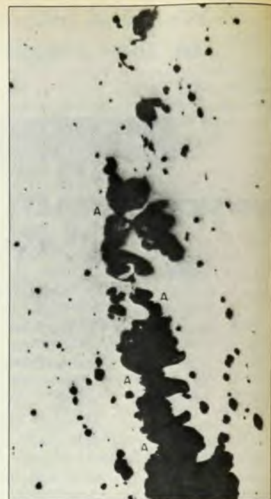
A partial spall (dynamic rupture) is formed by the coalescence of voids in an aluminum plate of commercial purity. The photo on the left represents a width of about 5.0 mm; the tip of the crack is shown on the right at ten times higher magnification. Failure by void coalescence due to necking of the region between the voids in apparent near points marked "A."
