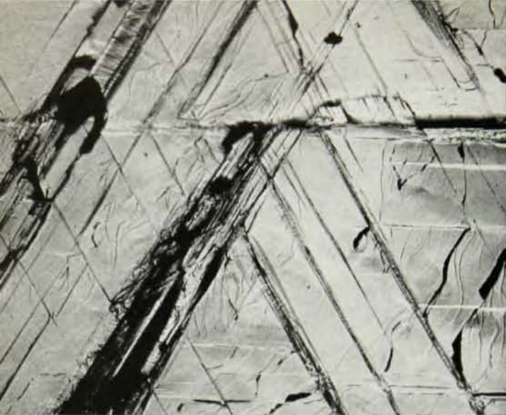
Figure 2. Fractograph—or photomicrograph of an unpolished and unetched fracture surface—for metallic bismuth, showing geometric markings which contain the story of deformation and fracture. Magnified 45 times.
