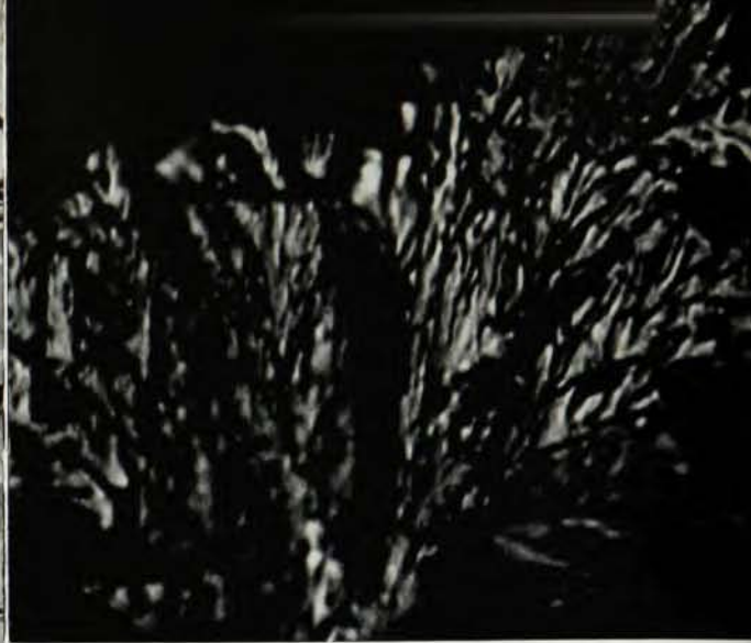
Figure 3. Fractograph of a tough steel suitable for such construction as ship plate. The individual grain is very small, causing fracture to change its path much more frequently as it jumps from grain to grain; and the microscopic path through the grain itself is rough and torturous, as illustrated visually by this coral-like pattern of toughness. Magnified 1250 times.
