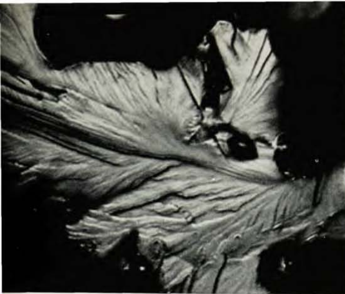
Figure 4. Fractograph of a steel which, in contrast to that in Figure 3, lacks toughness and is unsuited for such applications as ship plate. The facet of this individual grain is comparatively smooth, showing much less interruption of the progress of fracture than in the previous figure. Magnified 1250 times.
