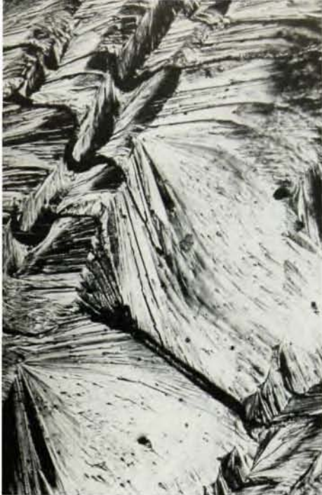
Figure 6. Fracture passing through a grain of molybdenum reveals a remarkable pattern which is probably the frozen record of the story of solidification and growth. Magnified 130 times.
