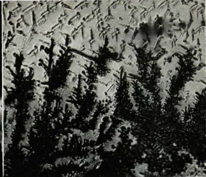
Figure 5. Unique fractograph of a molybdenum metal showing the exterior surface of a grain—the grain boundary—with two intruding growths which strongly affect the forgeability. The upper field has feathery forms which carbides necessary for forgeability. The lower field has a weedy-looking growth of oxide, caught in the act of invading the carbide area to form carbon ox gas which is removed by the vacuum treatment. The oxide growth causes grains to fall apart, preventing forging. Magnified 385 times.
