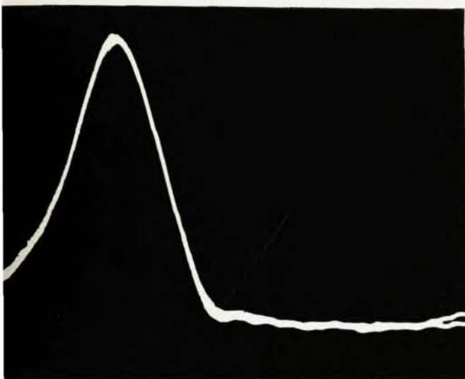
These nuclear induction signals are from protons in water in which is dissolved a slight amount of manganese sulphate to accelerate the establishment of thermal equilibrium. The illustration on the left represents a dispersion signal, that on the right an absorption signal. One obtains one or the other (or some intermediate signal) by adjusting the phase component of the observed signal with respect to the driving radio-frequency field.
