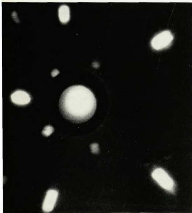
Neutron Laue pattern of rock salt (above) and of lead (below). The lead was five-eighths of an inch thick!
