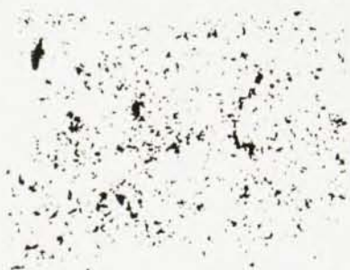
Typical area of nuclear emulsion exposed to a beam of mitibules, showing that the mitibule leaves no track and therefore is probably uncharged.
