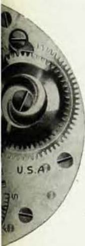
The plates and bridges of this watch have been made of plastic so that the entire train may be clearly seen.
