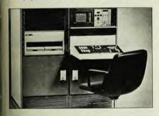
and X-Y plotting tasks. Since both processors use direct memory access, the load on the Central Processor is reduced to a minimum. The entire family of PDP-11's from D.E.C. is available for use as the SCORPIO central processor unit. By using a secondary UNIBUS for the time critical functions—data acquisition and display—the primary UNIBUS and PDP-11 CPU are essentially devoted to data analysis and computation—Canberra Industries, 45 Gracey Avenue, Meriden, Ct. 06450.
