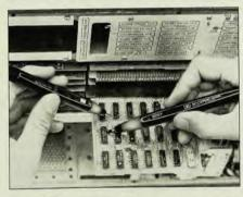
stimulates circuits for stimulus–response testing. A feature of the pulse is its ability to supply pulse streams of 1, 10, or 100 Hz, or bursts of exactly 10 or 100 pulses, as well as single pulses. The current tracer senses logic current pulses as small as 1 mA up to 5 mm from the conductor. It operates on all logic families having current pulses from 1 mA to 1 A with repetition rates to 10
