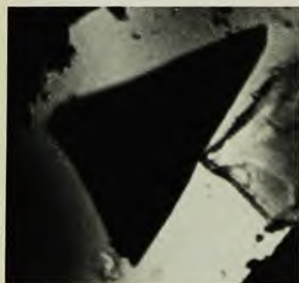
A single crystal of zinc sulfide at 150 kbar in the diamond cell is transformed, in this sequence, to a black opaque phase, which is electrically conducting. The adjacent object is a crystal of ruby that acts as the pressure sensor. The Inconel gasket, which measures approximately 0.5 mm along its major axis, contains the pressure transmitting fluid. Figure 4
