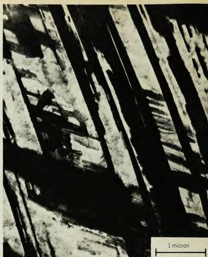
That on the right had been cold worked; it shows thick films on martensite platelets. These transmission electron micrographs show the films after the metal was dissolved away. Figure 3
