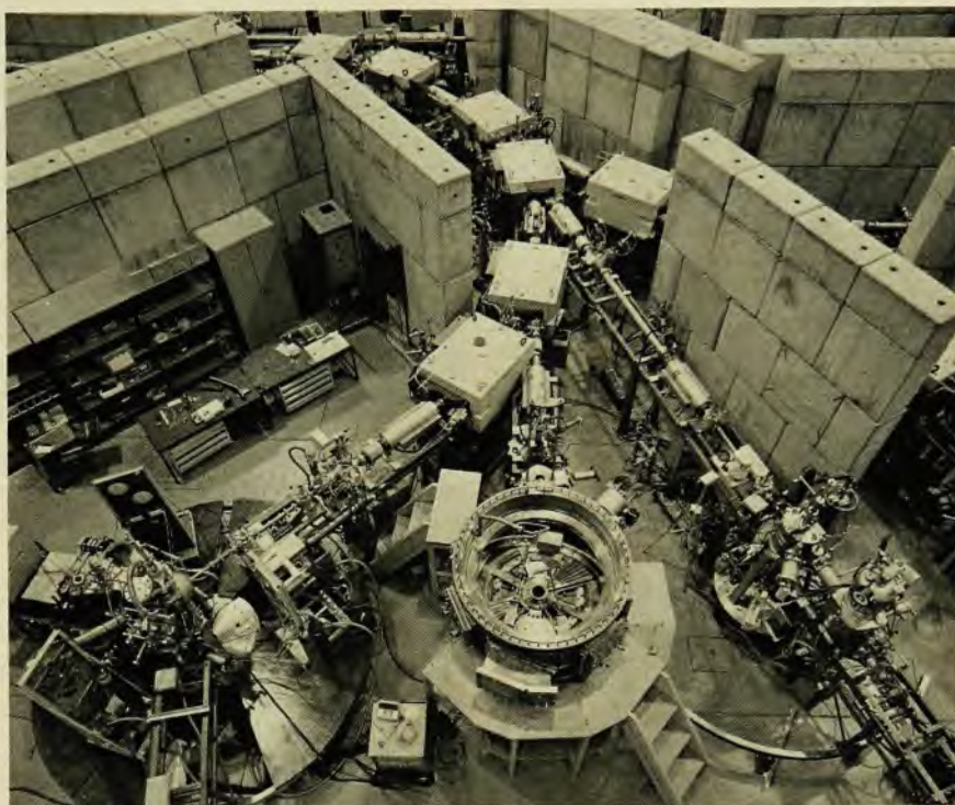
Scattering-chamber area at GSI, the heavy-ion facility near Frankfurt. In left foreground is kinematic coincidence spectrometer with two position-sensitive particle-detector telescopes. In center foreground is multi-purpose scattering chamber with 1.5-m diameter. In right foreground is scattering chamber for particle spectroscopy with time-of-flight and \Delta E - E spectrometers.
