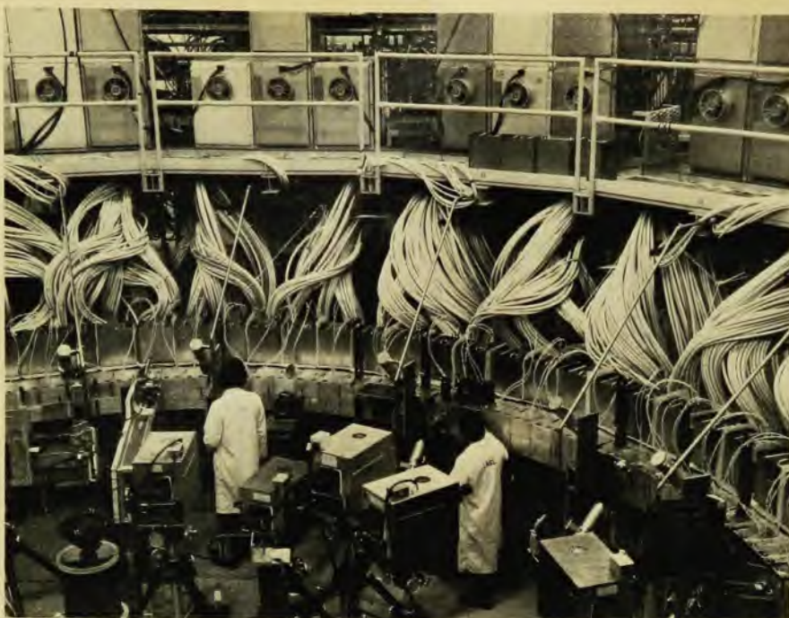
Scyllac compression coil. Image-converter cameras (foreground) take streak photos of plasma through slots in front and top of coil. Five optical feedback detector stations are shown. Bundles of white cables power compression coil from capacitor banks in rear (not shown).
