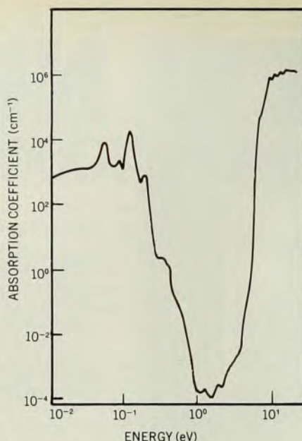
Absorption spectrum of a soda-lime silicate glass, obtained by combining measurements made on bulk glass in the high-attenuation regions with data from fibers in the low-loss regions. (From B. G. Bagley et al. , reference 4.)
