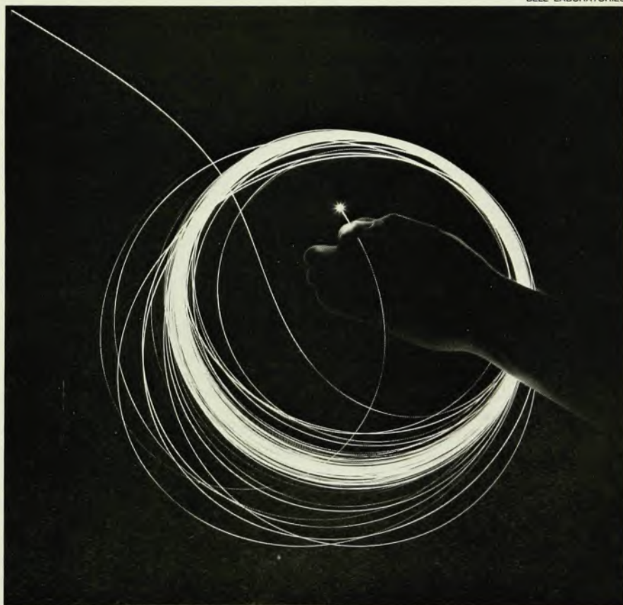
Conversation piece? Optical waveguides such as this glass fiber may carry your voice, digitally encoded, in the not-too-distant future. The fibers are strong, flexible and can be cabled together; light leakage at gentle bends is not a serious problem.
