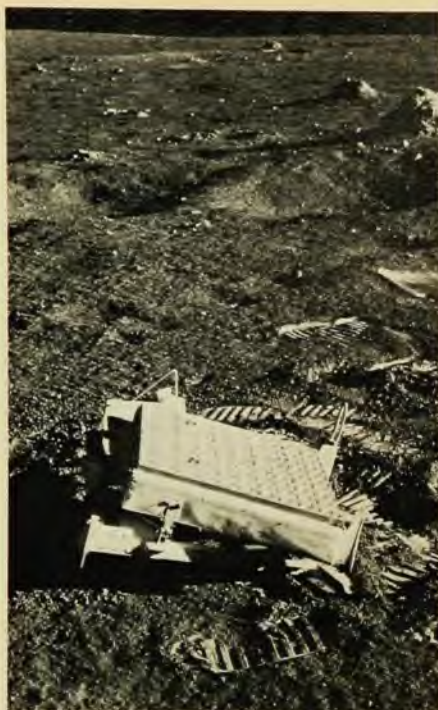
Lunar laser-ranging reflector package. This device, shown at Fra Mauro landing site, was installed by Apollo-14 astronauts. It contains 100 solid fused-silica corner reflectors mounted in a 46-cm square aluminum panel. Each reflector is 3.8 cm in diameter.
