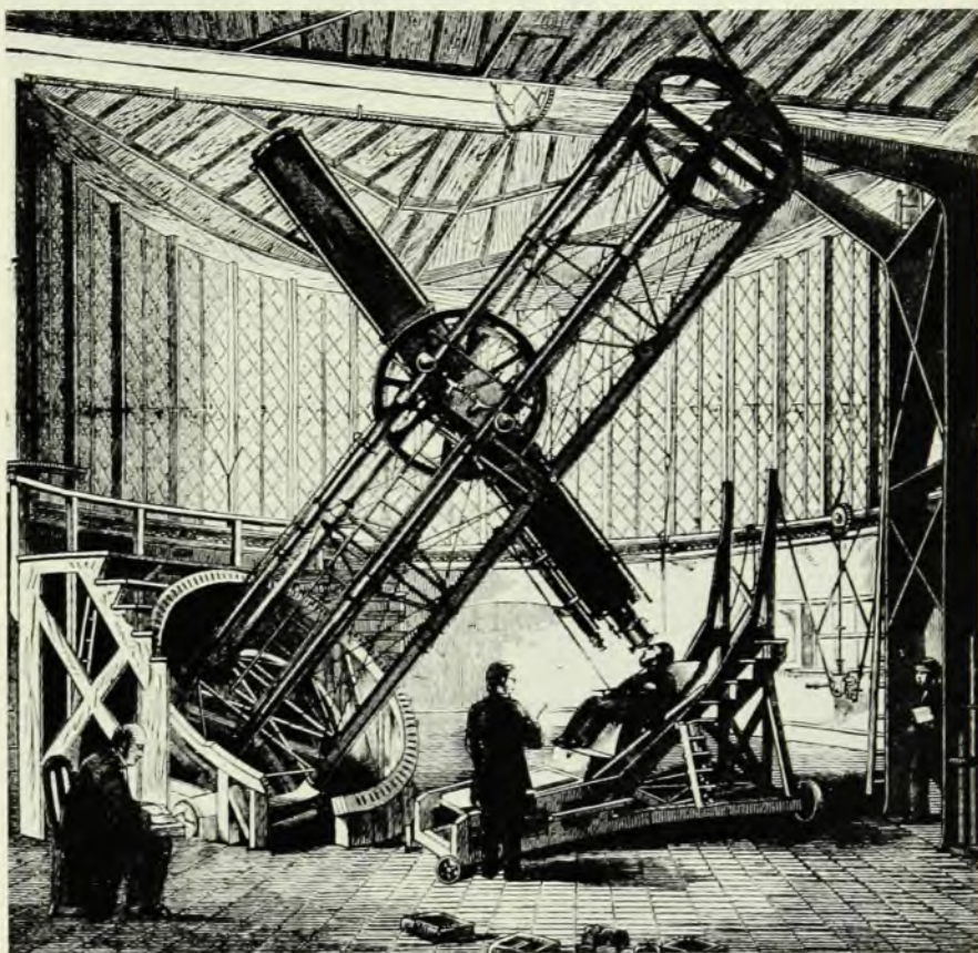
Equatorial telescope (12.8 inches) in operation at the Royal Observatory, Greenwich, in the 1860's. The engraving, from the 1880 edition of E. Dunkin's Midnight Sky , appears in volume 3.
