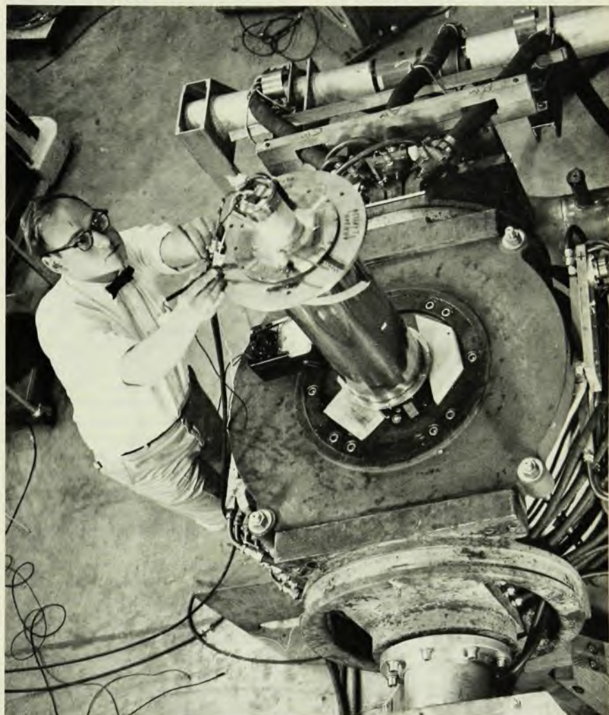
World's strongest direct-current magnet (22 Tesla) is used by experimenter Bruce Montgomery to make a low-temperature measurement. Photo by Francis Bitter National Magnet Laboratory.
