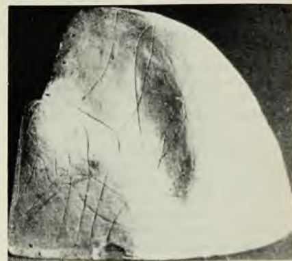
Model of the thermodynamic surface for water, presented to Gibbs by James Clerk Maxwell in 1875. It is now on permanent exhibit at the Gibbs Research Laboratory of Yale University. Maxwell's own copy of the model is at the Cavendish Laboratory of Cambridge University. Such equilibrium surfaces help clarify thermodynamic relationships. (Photo: Yale) Figure 1
