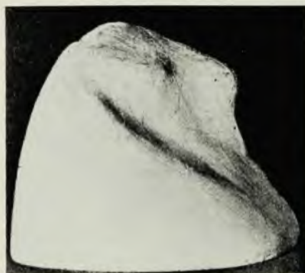
Model of the thermodynamic surface for water, presented to Gibbs by James Clerk Maxwell in 1875. It is now on permanent exhibit at the Gibbs Research Laboratory of Yale University. Maxwell's own copy of the model is at the Cavendish Laboratory of Cambridge University. Such equilibrium surfaces help clarify thermodynamic relationships. (Photo: Yale) Figure 1
