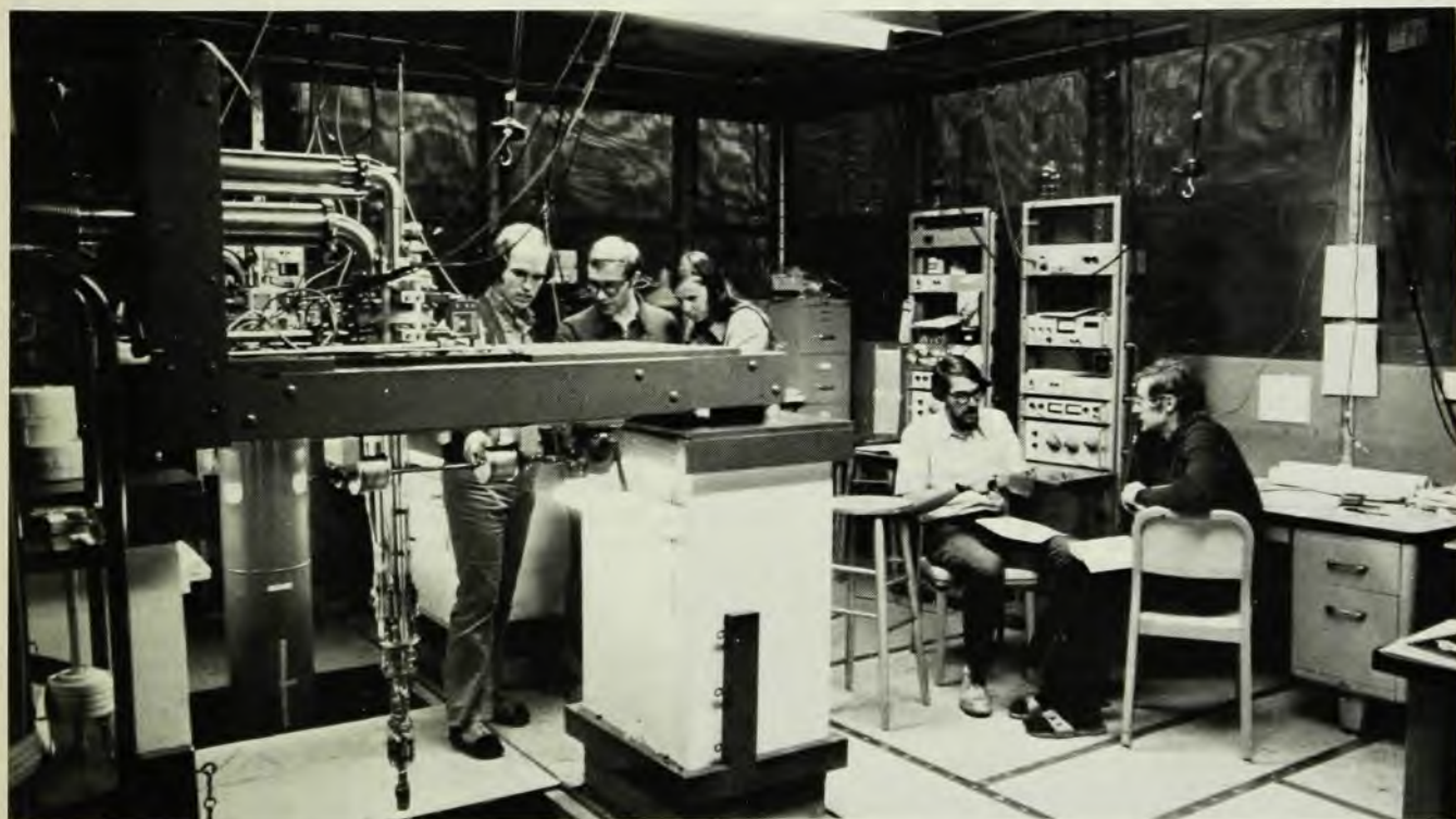
A dilution refrigerator with its pumping lines emerging above (left foreground) hangs over an open pit in Wheatley's copper-screened lab. Another one (behind it and to the left) is enclosed in its Dewar.
