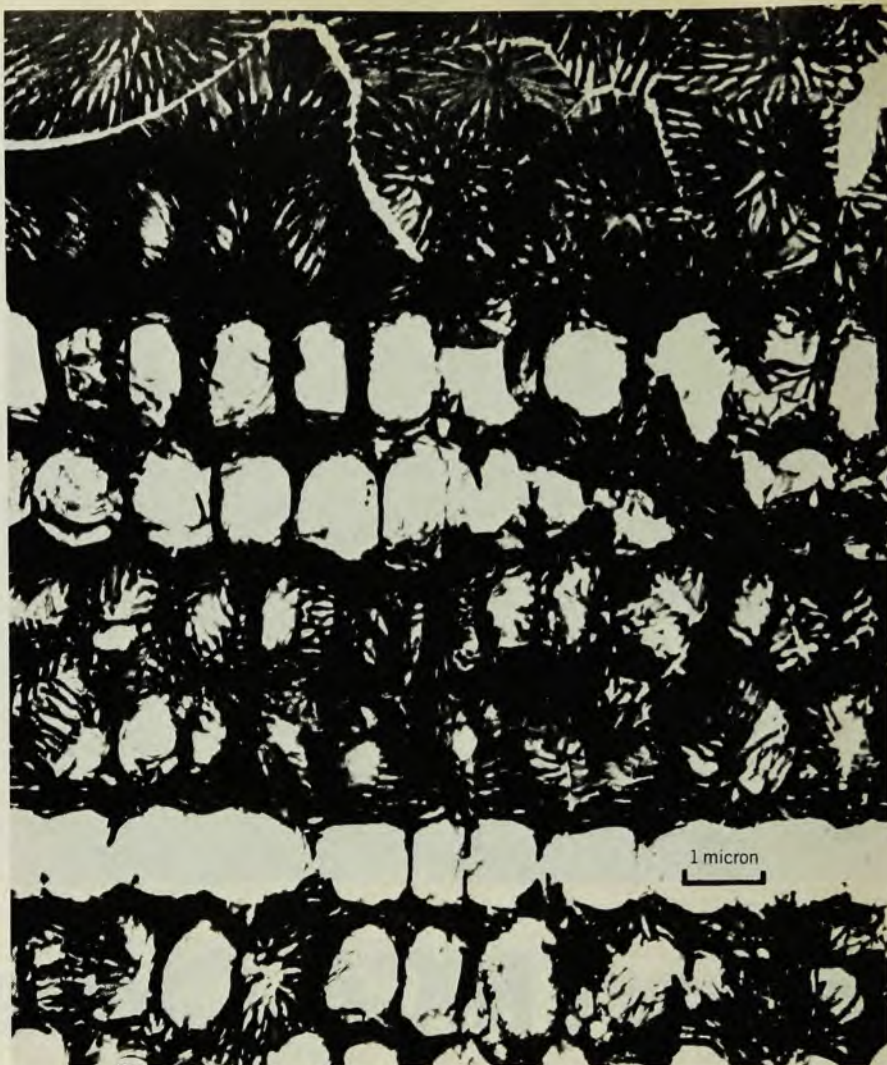
An extraction replica of the region of the CoTaC-3 alloy shown in part c of figure 6. This transmission micrograph shows a dendritic solid solution and a fine eutectic. Figure 7
