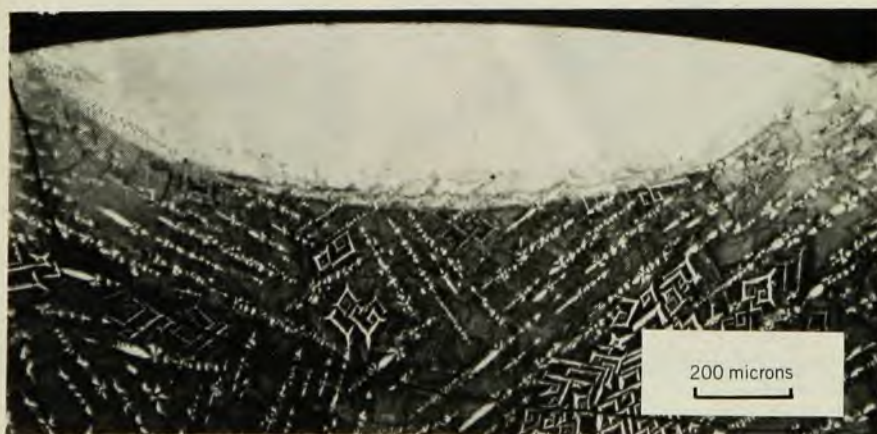
Light micrograph of a laser-glazed sample in transverse cross section. The alloy, of palladium with 4.2% copper and 5.1% silicon, is normally crystalline. Because of the rapid chilling characteristic of the laser glazing process, however, the part in the laser pass is amorphous; this was verified by electron diffraction and observation of the fracture surface. Figure 3
