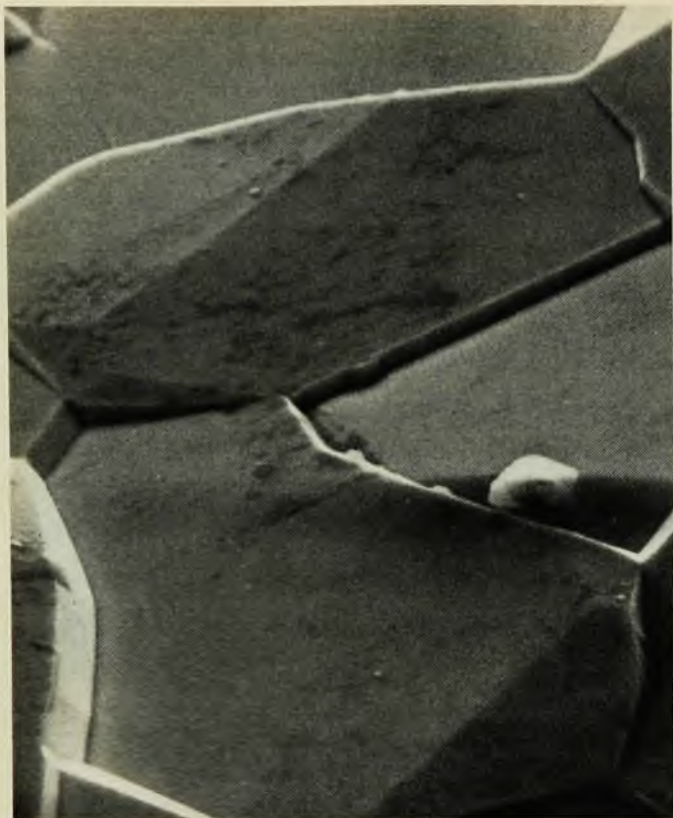
The surface of titanium , shown at a magnification of about 1000 in this scanning electron micrograph, reveals its grain boundaries. The specimen was thermally etched. Because of its great depth of field and range of magnifications, the SEM technique has many applications. (After M. Meshii and others, Northwestern University.) Figure 9
