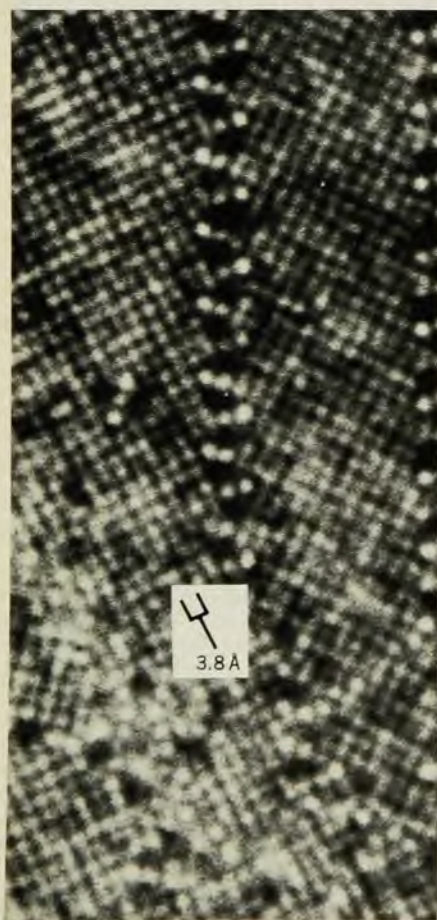
High-resolution electron micrograph of a crystal of 4\text{Nb}_2\text{O}_5 \cdot 9\text{WO}_3 , showing the nucleation of a disordered tetragonal tungsten-bronze-type structure at twin boundaries of the near-cubic \text{WO}_3 -type phase; large white spots are pentagonal tunnels. (Photograph by S. Iijima, Arizona State University.) Figure 7
