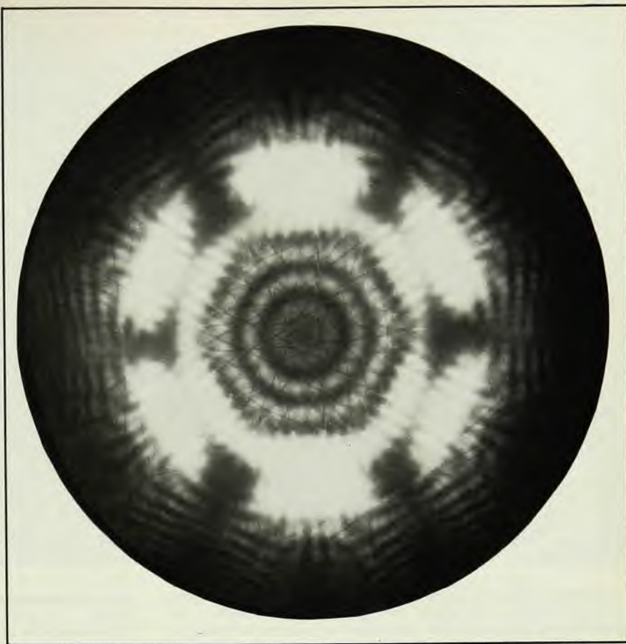
Convergent beam pattern from silicon [111] zone axis, taken with 200-kV electrons, reveals a mesh of higher-order K lines (Kikuchi in electron, Kossel in x-ray, diffraction) of fine angular diameter. (After G. M. Rackham and J. W. Steeds of Bristol University.) Figure 8
