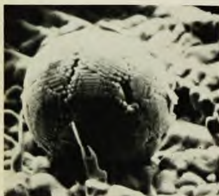
Scanning electron micrograph of a microsphere on the surface of a hot crack of a weld in Ni 200 alloy. The sphere diameter is 50 microns. Note the dendritic structure indicative of the thermodynamic conditions when the sphere was formed. (Reference 12.) Figure 5
