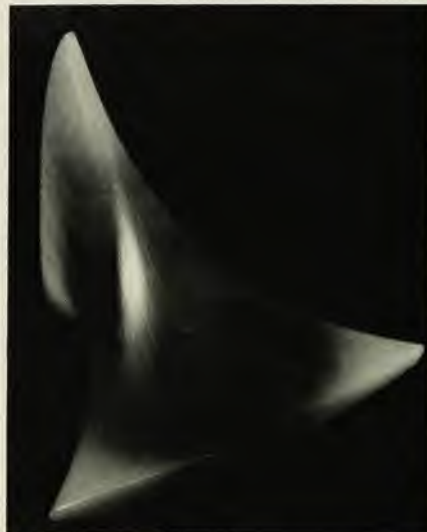
The magnetic field produced by a "baseball seam" coil for plasma containment. (Model, Lawrence Radiation Laboratory.)
