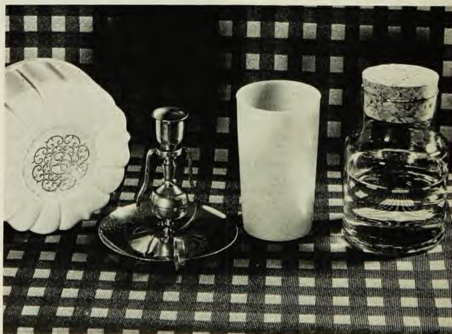
Four classes of objects. Left to right, the plastic box shows diffuse reflection, the candleholder specular reflection. Diffuse and specular transmission are seen with the tumbler and glass jar.
