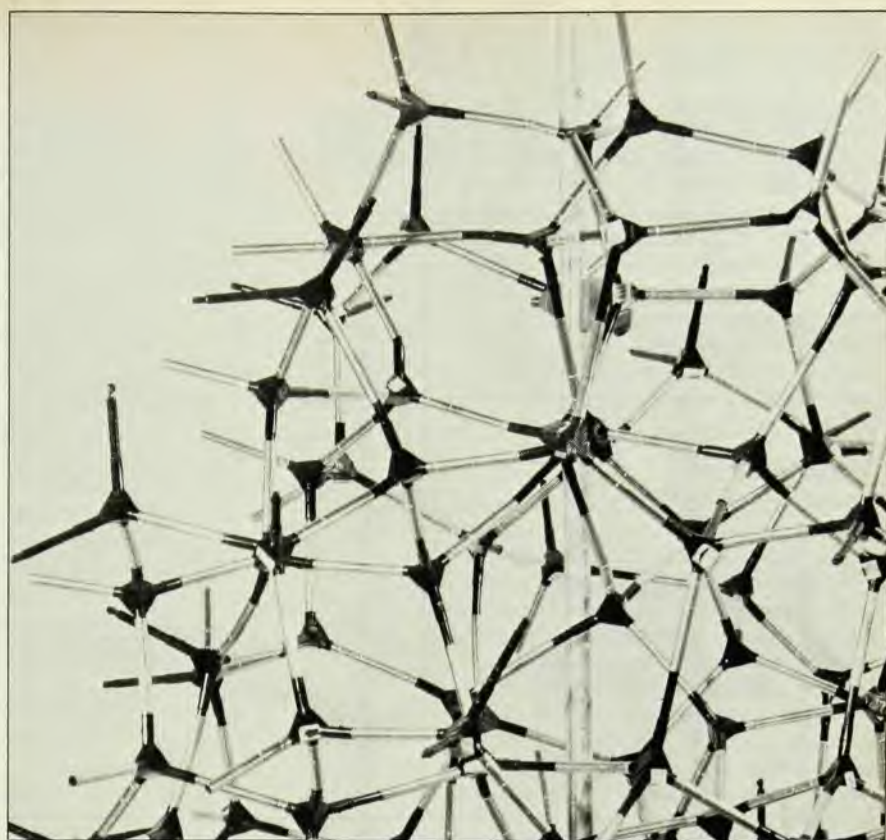
A model of the structure of amorphous germanium or silicon. In addition to the sixfold rings typical of the diamond structure, fivefold and sevenfold rings are evident as well. (Photo courtesy of G. A. N. Connell, Harvard University.)
