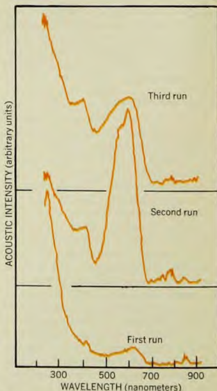
Photoacoustic spectra of Cooper blue. The photosensitive material was dark-adapted before the lower spectrum was made. The middle spectrum was run afterward, and then the upper spectrum, with only a few minutes separating the runs. Figure 8
