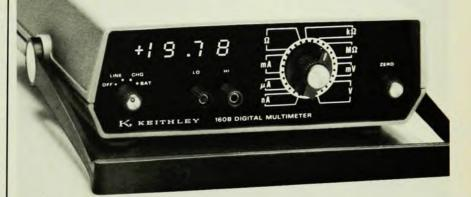
**The Model 160B.** It's the epitome of a DMM for scientific and engineering labs. Sensitivities down to 1 microvolt, 10 picoamps, and 1 milliohm are founded on Keithley's lifetime of expertise in designing and building low-level instrumentation.
