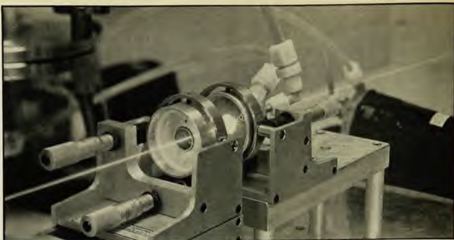
The first continuous organic dye laser, tunable in the 5500–6500 Å range, operated at the Kodak Research Labs in 1970. Pump light enters and is focussed into the dye-laser cavity
