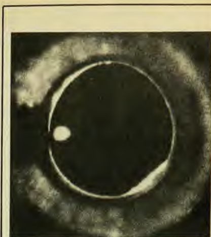
Electron-hole drop in germanium has been photographed for the first time by a group at the University of California, Berkeley, and the Lawrence Berkeley Laboratory. The drop was formed by applying a nonuniform stress to a single crystal of germanium (seen as a disc in the photo). When an Ar-Kr laser is focused onto the crystal, a single large electron-hole drop (the bright ring at the left) forms at the point of minimum drop energy. The photo was obtained by focusing the 1.75-micron recombination luminescence onto a lead-salt photoconductive surface (a vidicon tube). Drop lifetime is about 490 microsec. The existence of electron-hole drops was first proposed by L. V. Keldysh in 1968 to explain a sharp increase in the photoconductivity of germanium, and smaller droplets have been produced experimentally before the Berkeley work. The Berkeley group includes James Wolfe, William Hansen, Eugene Haller, Robert Markiewicz, Charles Kittel and Carson Jeffries. This photo first appeared in Phys. Rev. Letters 34 , 1252 (1975).
