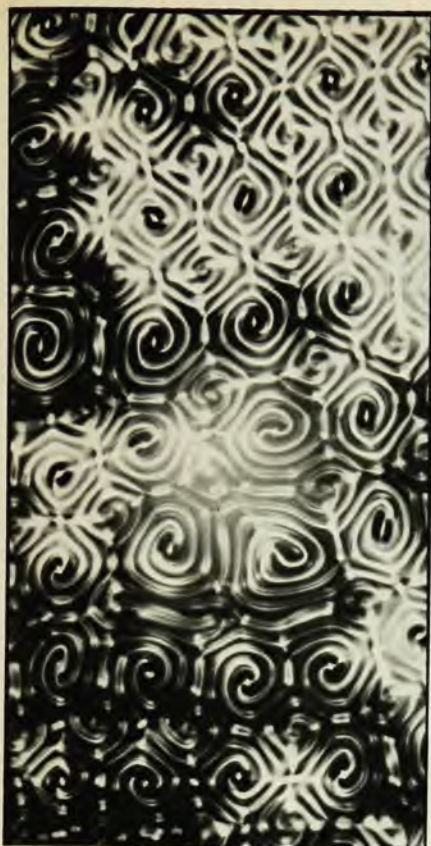
A cholesteric liquid crystal will show its "fingerprint" or "focal conical" when subjected to a low frequency, medium-strength electric field. The photograph is from the Laboratoires d'Electronique et de Physique appliquée, the French member of Philips Research Labs.
