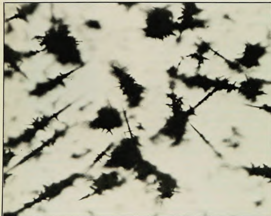
Etched olivine crystal from a stony-iron meteorite. The long tracks are due to ultraheavy cosmic rays ( Z > 30 ). The densely clustered short tracks are those of iron nuclei ( Z = 26 ); they are visible only near their intersections with tracks of ultraheavies. Nuclei lighter than iron do not produce etchable tracks in these crystals. Photo: D. Lal. Figure 2
