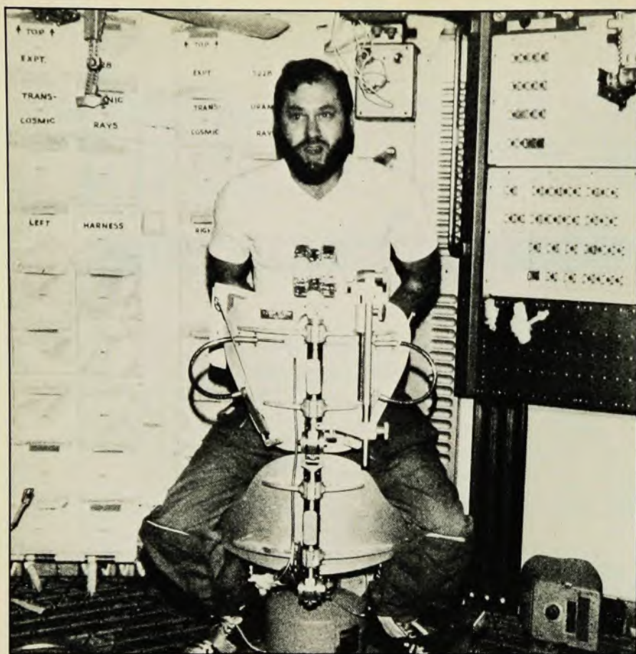
Inside the Skylab orbiting workshop during a space mission, bearded astronaut Bill Pogue sits in front of the array of detectors of ultraheavy cosmic rays that line the thin outer wall of the craft. Each of the 36 white cloth packets (some are marked "Transuranic cosmic rays") contain an 18 cm X 20 cm X 1 cm stack of Lexan plastic. NASA photograph. Figure 1
