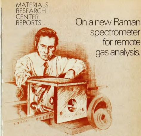
At the Materials Research Center, Dr. J. J. Barrett has been investigating methods for the remote analysis of gases at low concentrations (ppm). These studies have led to the development of an instrument system that sensitively measures light which has been scattered from a gas by the rotational-Raman effect.
