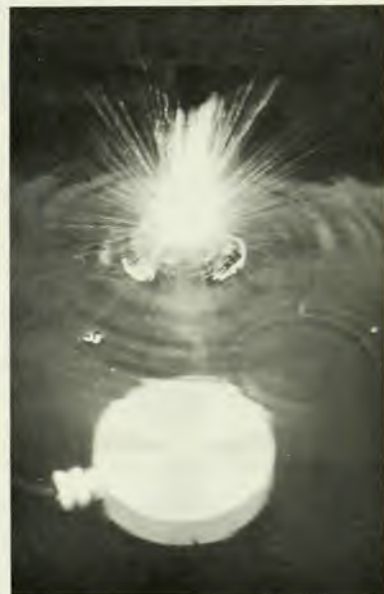
Collision of a 500-watt pulse at 500 kHz with the water's surface. The transducer is a standard 1000A, as delivered. It is at a depth of 25cm, with its face parallel to the water's surface.
