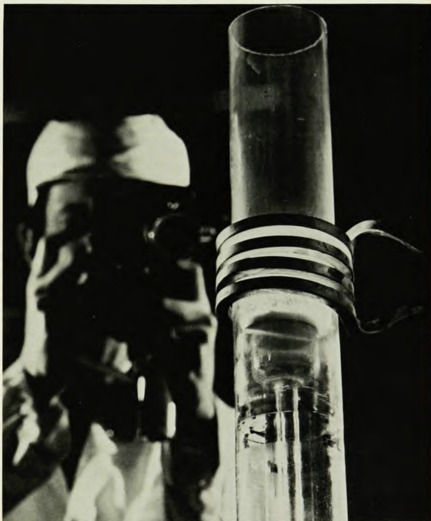
Ultra-pure glass is melted in a radiofrequency field by direct coupling with a water or gas-cooled crucible. This technique for melting batch materials, developed at Standard Telecommunication Laboratories in the United Kingdom, eliminates contamination by crucible degradation.
