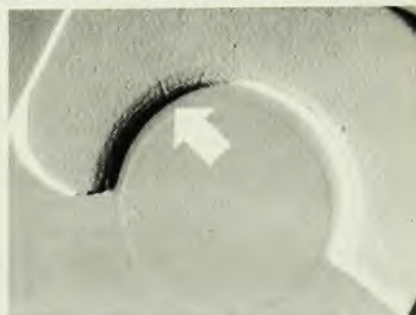
Same Radiograph edge-enhanced clearly shows radial crack.
