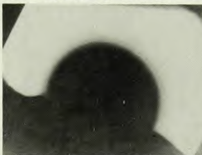
Radiograph of pin-jointed lug. (Photo courtesy of Magnaflux).
