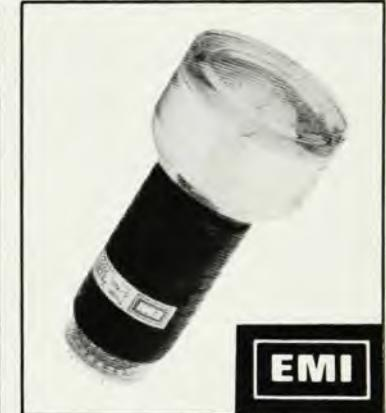
EMI has added a 3" linear focused tube to its range of  $\frac{3}{4}$ " and 2" tubes. The unique 9821 incorporates a computer designed front end to ensure maximum collection efficiency. Fitted with 12 dynodes having BeO secondary emitting surfaces, the 9821 gives a typical gain of  $4 \times 10^7$  at 2800 volts. The high efficiency bialkali cathode also ensures a low dark current level (typically 3 nA at 200 A/lm) required for certain applications.
