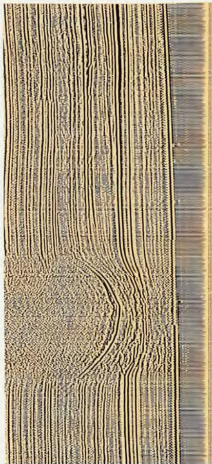
This seismic reflection record from a deep-water survey reveals the probable existence of a salt dome (bottom of record).
