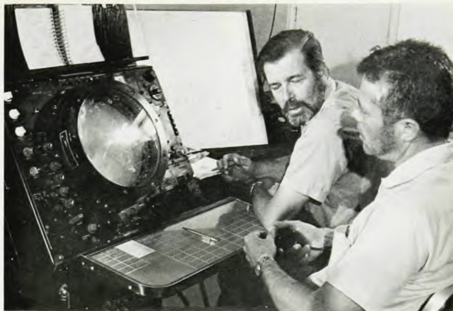
Moisture-searching radar is used at the National Center for Atmospheric Research to find hail-producing storms as part of the North-East Colorado Hail Experiment. (NCAR photo.)
