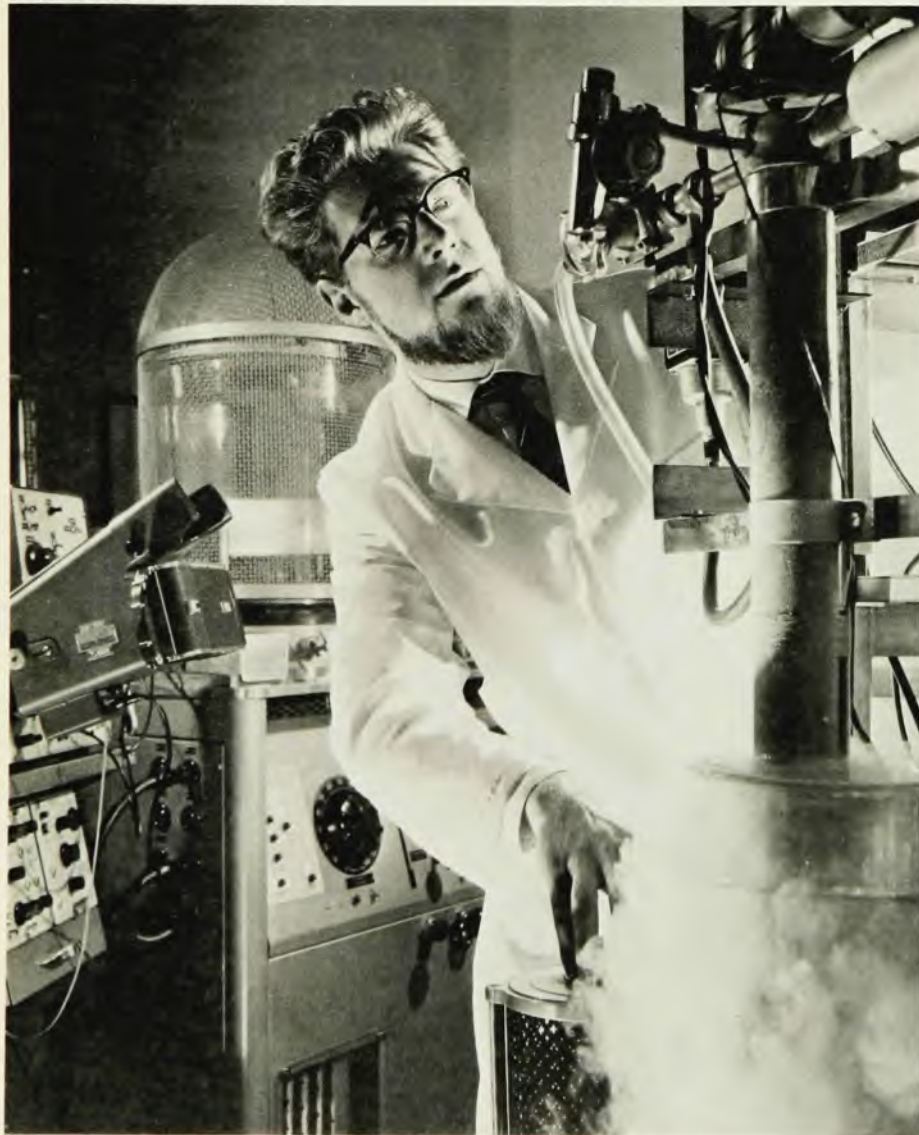
Measuring the glow curve of a semiconductor device. To develop new products, physicists in telecommunications laboratories explore materials that exhibit potentially applicable effects.
