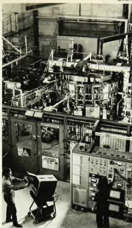
European fusion research is coordinated with the world effort. This view of the CLEO Tokamak at Culham Laboratory shows the toroidal plasma confinement device in the background, with diagnostics area in foreground.
