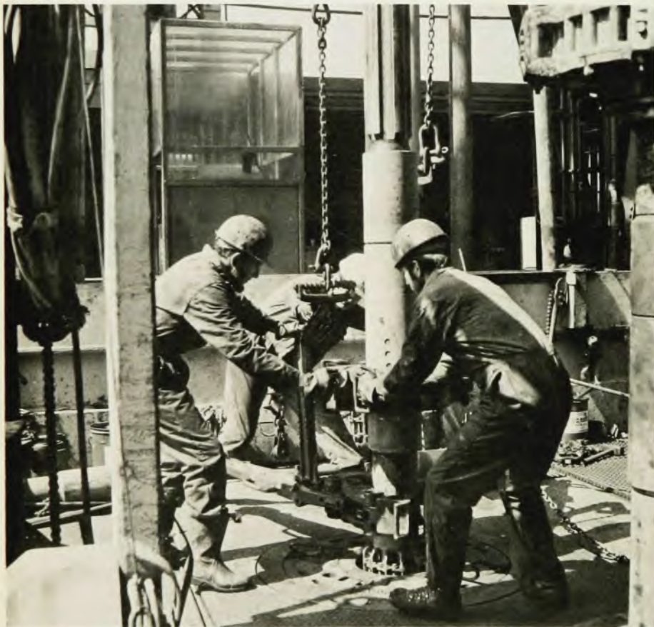
Offshore oil drilling in the Celtic Sea. These men are inserting a "bumper sub," which compensates for the motion of the vessel, into the drilling string. The Nordic Offshore Drilling Company's Havdrill , which is on long-term charter to British Petroleum, is drilling a "wildcat" well.
