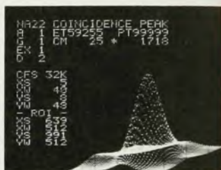
2. 4420 isometric display of 35x40 data point region of interest for detailed spectrum analysis in dual parameter study. Resolution—4K x 4K data points.
