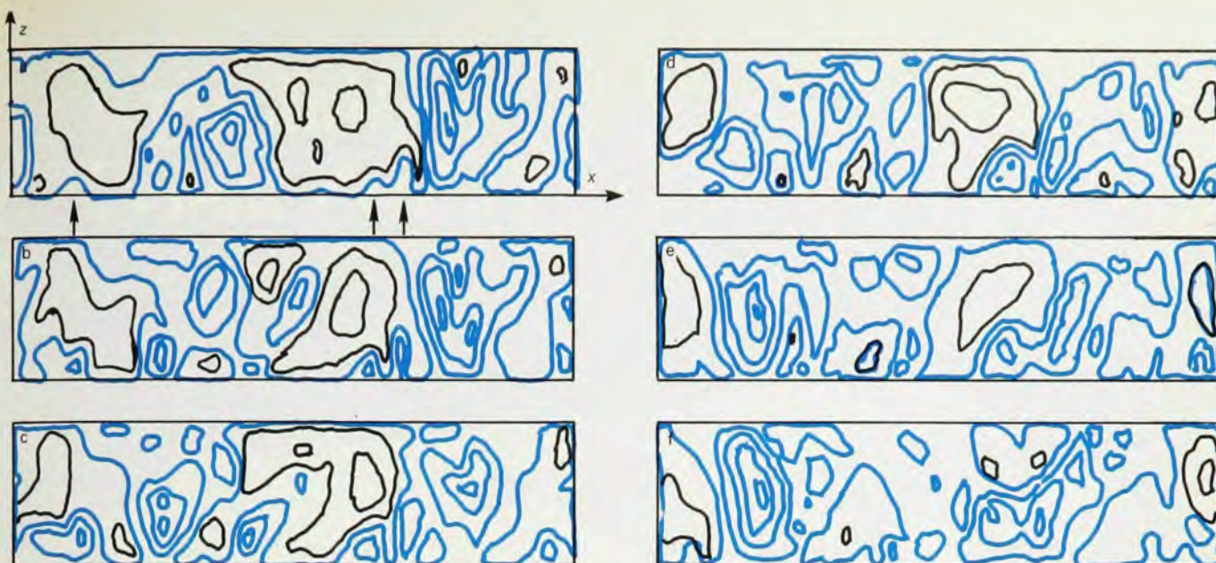
Time sequence of the vertical velocity field in an extremely large computer simulation of boundary-layer turbulence by J. W. Deardorff (reference 8). Black lines are contours of updrafts and the colored lines are contours of downdrafts. Note the three
