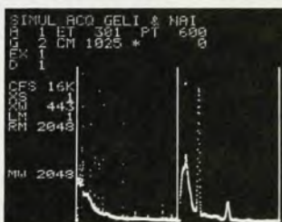
1. 4420 display showing spectra acquired simultaneously from GeLi detector in 4096 channels and NaI detector in 1024 channels.
