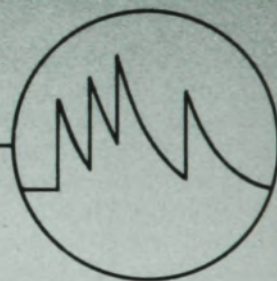
Random Mode. High count rate showing pile-up
