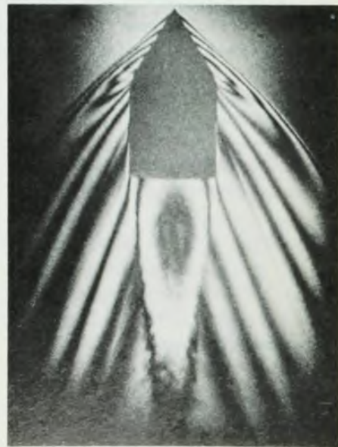
A laser hologram produced this image of a 22-caliber bullet travelling at Mach 2.5.
