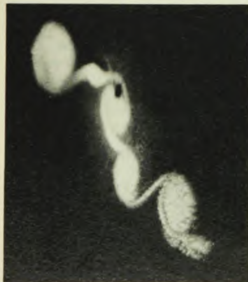
A clockwise vortex structure forms in a laboratory electron sheet beam (left). A model developed by Webster and Hallinan may serve to explain this pattern and one of similar appearance in aurorae (right). This example was recorded by a low-light TV camera.
